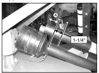
Figure 4. Determine Shield Length
